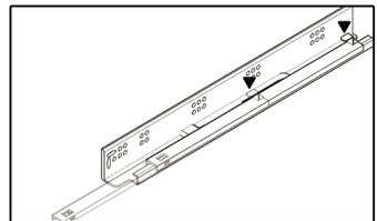
Picture shown is the complete set of the drawer glide. Part shown as semi-transparent indicates this object is movable, which will help in identifying in the following step.
