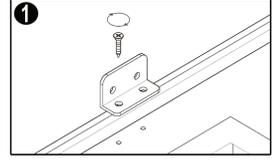
► Place the face frame in a face down position to a flat surface. Secure the L-Shape connector clip with 1/2" Philips screws to the pre-drilled holes # 1
