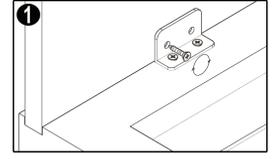
► As show in this picture, slide the side panel into the face frame's groove located on the left or right. Then, secure the side panel to the L-shape connector clip # 1 using 1/2" Philips screws .Repeat this step for the other side panel
